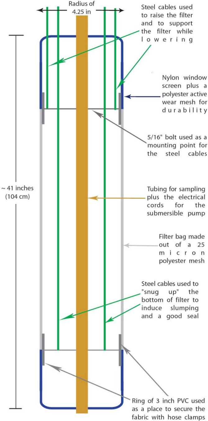
**Appendix Figure D- 3: Picture of the actual filter tested in the field. This photo was taken at the end of the field test.**
