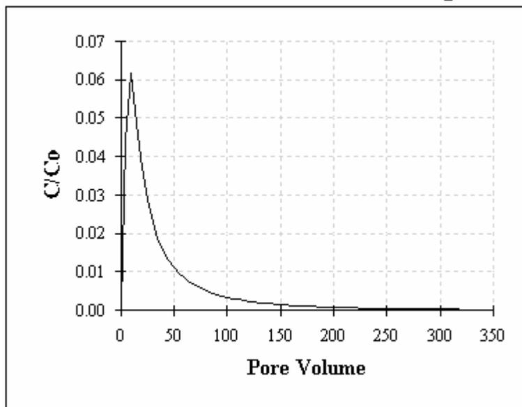
Figure 4: Predicted breakthrough curve for cationic SMZ.
