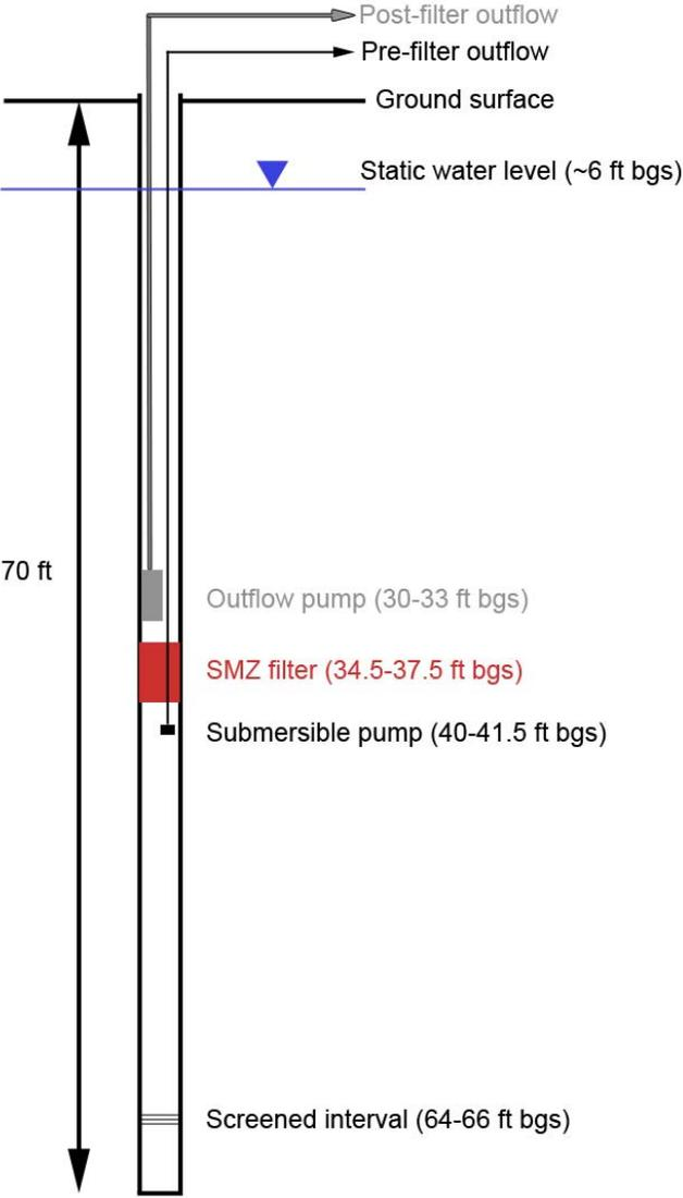
**Appendix Figure D- 2: Diagram depicting the construction of the filter prototype tested in the field.
