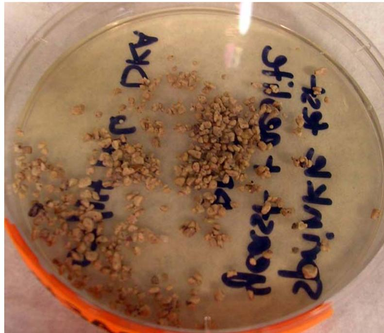
Appendix Figure A- 3: Hydrophobic SMZ with minor yeast growth on an agar plate.
