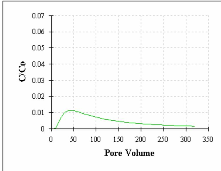
Figure 5: Predicted breakthrough curve for hydrophobic SMZ.
