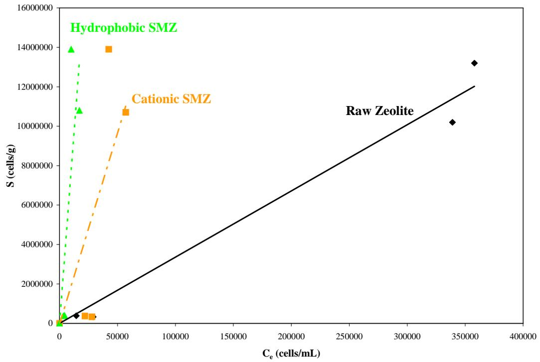
**Figure 2: Linearized Freundlich isotherm for *S. cerevisiae* and three zeolite treatments (raw, cationic, and hydrophobic SMZ), based on the batch experiment results.**
